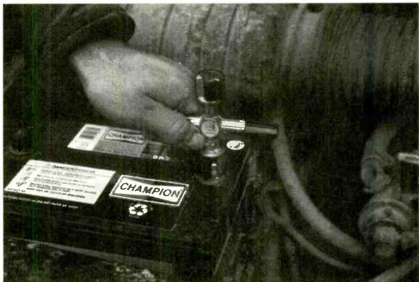
Fig. 3. If the battery terminals are corroded from the acid fumes that can be released by the battery, a simple battery-post brush will clean them up.
