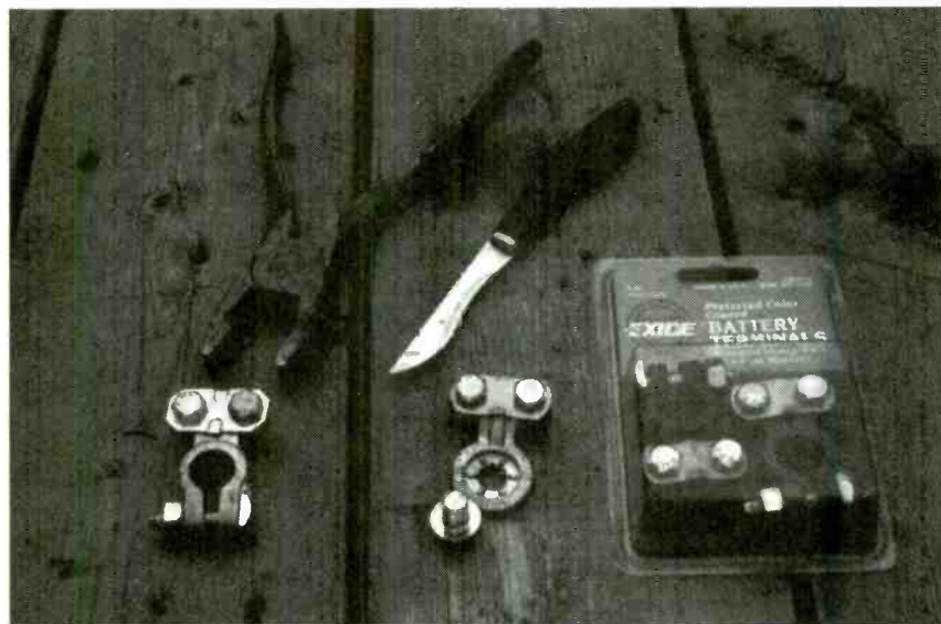
Fig. 4. In an emergency, you only need a knife and a pair of pliers to do a roadside replacement of a damaged or corroded battery clamp.
