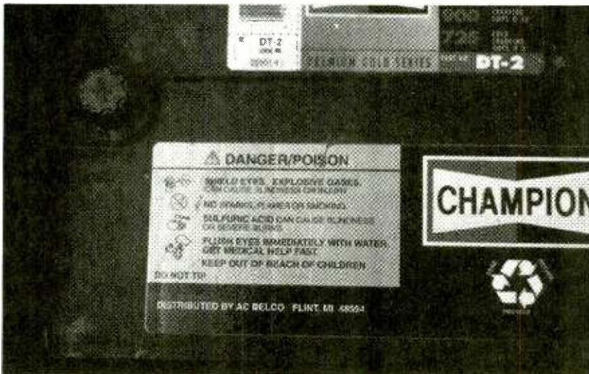
Fig. 2. Lead-acid batteries are constantly charged while the engine is running. That charging causes electrolysis to take place in the acid solution, producing hydrogen gas. Hydrogen gas is extremely explosive—any sparks or flames should be kept away from the battery at all times.
